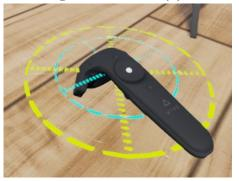
(e) Command to turn the drone to the left. Angular speed is proportional to the angle between controller's axis and forward vector of origin pose.
