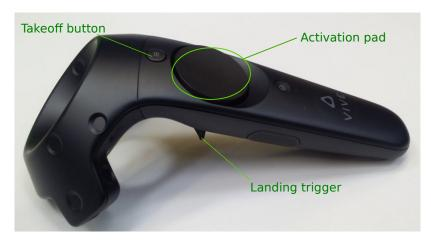
Figure 3.3: Layout of buttons on the motion controller used in our application. The activation pad is a touch sensitive sensor which can detect whether the user is touching it - without need for a strong press. Movement commands will only be sent while it is being touched.
